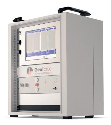
Icontrol combines the depth information with the obtained CPT data and provides power to the Icone. Icontrol is connected to a PC or Laptop with an USB-connection. The Ifield software package is installed on the PC or Laptop for on-line presentation on screen and recording of the CPT data. Icone and Icontrol work in conjunction with the usual equipment for depth registration and pushing.
